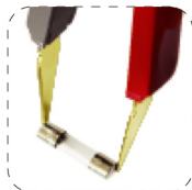
Fuse open & short check
